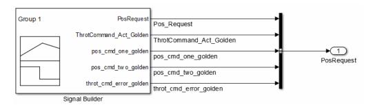
The subsystem uses a Signal Builder block for the test vector source. The block has data that drives the simulation (PosRequest) and provides the expected results used by the Verification subsystem. This example test harness uses only one set of test data. Typically, you create a test suite that fully exercises the system.
