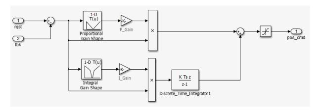
The PI controllers in the model are from a *library*, a group of related blocks or models for reuse. Libraries provide one of two methods for including and reusing models. The second method, model referencing, is described in "Simulation Test Environment" on page 2-8. You cannot edit a block that you add to a model from a library. You must edit the block in the library so that instances of the block in different models remain consistent.
