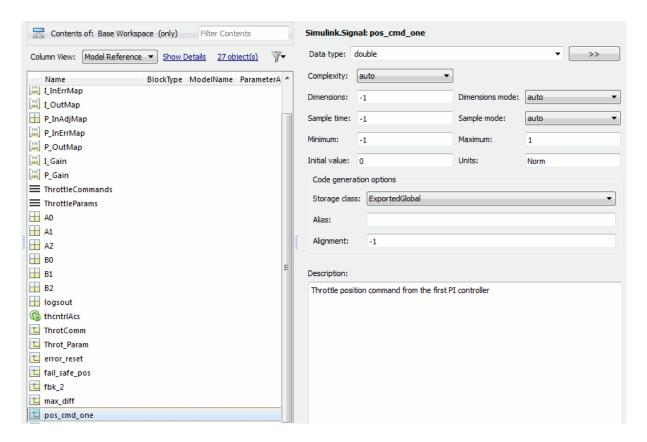
You can also view the definition of a signal object. In the MATLAB Command Window, enter pos cmd one:
