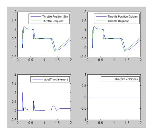
The lower-right hand plot shows the difference between the expected (golden) throttle position and the throttle position that the plant calculates. If the difference between the two values is greater than  $\pm 0.05$ , the simulation stops.
