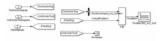
A test harness compares control algorithm simulation results against *golden data* — test results that exhibit the desired behavior for the control algorithm as certified by an expert. In the Verification subsystem, an
