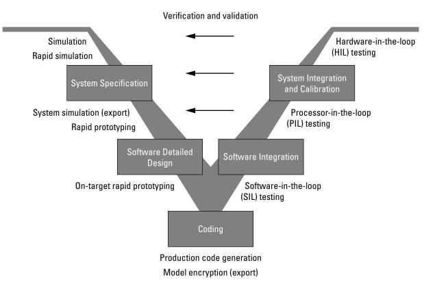
Depending on your application and its role in the process, you might focus on one or more of the steps called out in the V-model or repeat steps at several stages of the V-model. Code generation technology and related products provide tooling that you can apply at each step.
