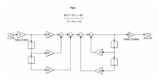
The Plant subsystem models the throttle dynamics with a transfer function in canonical form. You can create plant models to varying levels of fidelity. It is common to use different plant models at different stages of testing.
